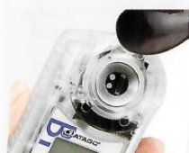
Apply 2 to 3 drops on the Prism surface.
