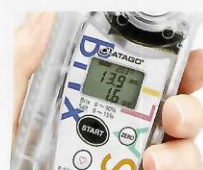
Measurement value and prism temperature are displayed in 3 seconds!
